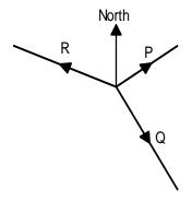
**P** is of magnitude 350N on a bearing of 060°, **Q** is of magnitude 600N on a bearing of  $\theta$ , where  $090^{\circ} < \theta < 180^{\circ}$ , and **R** is of magnitude xN on a bearing of 285°.
